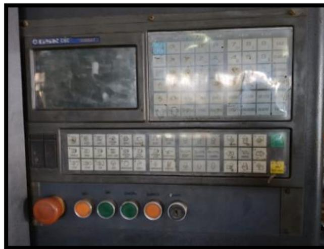
Gambar 22 Control GSK mesin Milling
